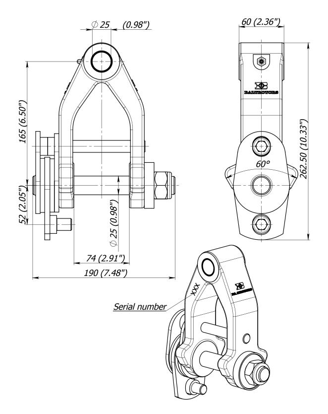
\* Pin locking nut is tightened with a torque of 60 - 160 Nm (45 - 120 lb ft) dependent on desired brake power.
