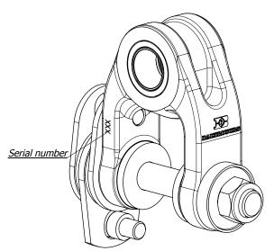
Pin locking nut is tightened with a torque of 60 - 160 Nm (45 - 120 lb ft) dependent on desired brake power. Weight - 6.5±1 kg (14.55±2.20 lb)
